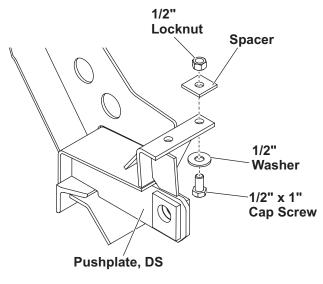
5. Tighten all fasteners at this time, according to the torque chart provided. Bend the cap screw handles out of the way.
