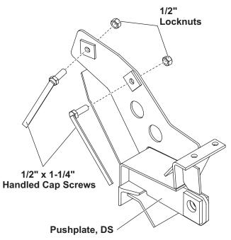
4. Using the pushplates as guides, drill a 17/32" hole up through the bottom of the bumper on the driver's side, and ream out the slot on the passenger's side, if necessary. Place a spacer above the holes on the inside of the bumper and secure with a 1/2" x 1" cap screw and 1/2" washer on the underside of the frame. Secure with a 1/2" locknut.
