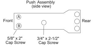
Install the 3/4" x 2-1/2" Gr. 8 cap screws in the center holes of the push assembly and through the slot in the A-frame from the outside. Install the 3/4" Gr. 8 flange nuts on the cap screws, finger tight. NOTE: For 9-1/2' EZ-V® blades, install blade stop kit 26634 before attaching angle rams.
