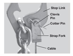
5. Insert the cable down through the hole in the strap fork. Attach the strap fork to the hole in the stop link on the lift arm with a 3/8" x 1" clevis pin and 1/8" x 1" cotter pin. Slip the cable thimble onto the top loop in the spring previously installed in the front of the A-frame.
