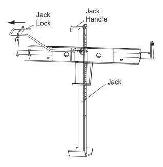
2. Align holes in headgear assembly with a hole in the A-frame pushears. Hole selection is determined by distance from center of the connecting pin hole to the ground. Refer to table below.
