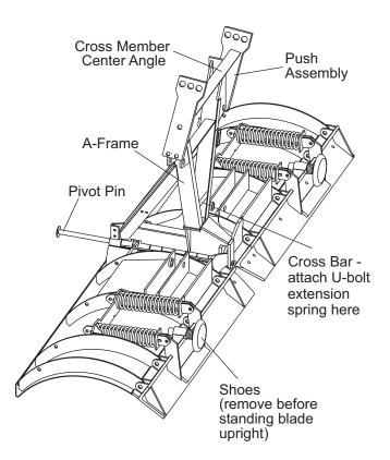
3. Install the push assembly to the outside of the A-frame ears with the flat side of the cross member center angle up.
