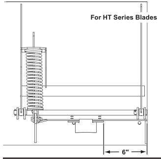
Position the shoe tube against the rear edge of the base angle. Make sure the shoe bracket is parallel with the base angle.
