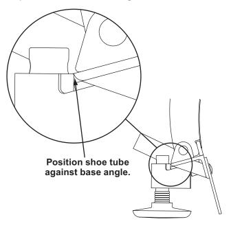
3. Using the bracket as a guide, drill four 17/32" holes in the base angle. Fasten with four 1-1/2" screws and 1/2" locknuts. Tighten to 115 ft-lb.
