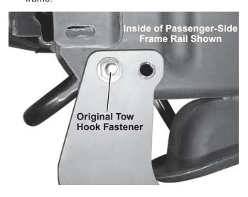
2. Rotate the passenger-side mount plate back, and push it tight up against the bottom of the frame. Clamp the mount plate in place against the frame.
