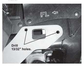
8. Insert two 3/8" x 1-1/4" cap screws with handles and 3/8" flat washers into the inside of the truck frame and out through the rear drilled holes.
