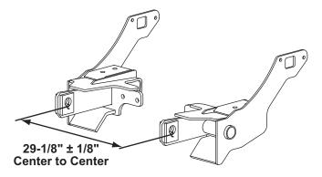
12. Tighten all fasteners according to the torque chart after achieving the appropriate dimensions.
