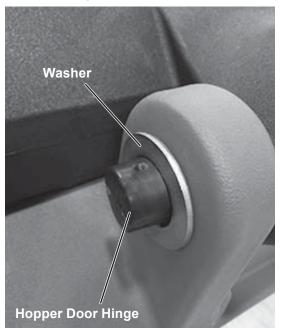
5. Using a power drill and 3/8" bit, drill a hole down through each of the door hinges, ensuring that drilling creates a hole on the top, and a hole on the bottom of the hinge.
