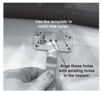
5. Drill out the holes marked In Step 4, creating four new rivet holes.
