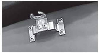
9. Verify that the hopper lid latch fully engages the new bracket and securely latches the lid in place.
