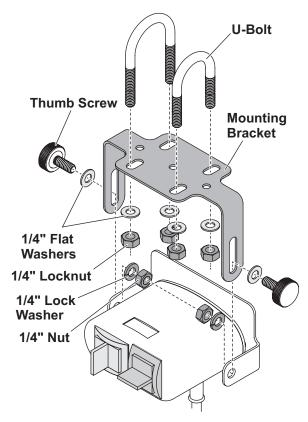
2. Attach the control to the slots in the bracket with two 1/4" thumb screws, two 1/4" flat washers, two 1/4" lock washers, and two 1/4" nuts as shown.
