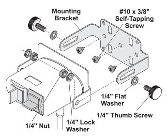
2. Attach the control to the slots in the bracket with two 1/4" thumb screws, two 1/4" flat washers, two 1/4" lock washers, and two 1/4" nuts as shown.
