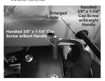
5. Bend the handles on two handled 3/8" x 1-1/4" cap screws as shown below. Insert the cap screw through the next access hole rearward and down through the bottom frame hole shown. Repeat for the other frame rail.
