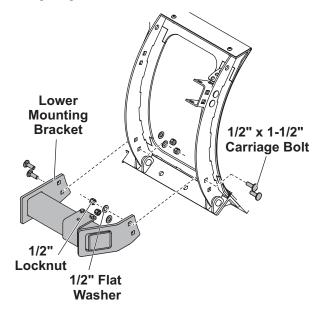
7. Insert the wing tube into the lower mounting bracket tube. Slide the wing into the tube until the stand pin holes in the wing assembly align with the corresponding holes in the mounting brackets. Install one of the 1/2" x 5-1/2" stand pins through the lower bracket hole.
