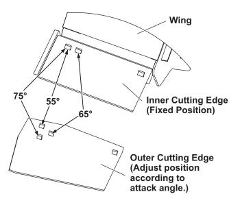
**HD2<sup>™</sup> Snowplow:** Align the holes in the cutting edges with the holes in the wing base angle that correspond to the 55° attack angle setting.
