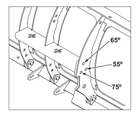
Align the holes in the cutting edges with the wing base angle holes corresponding to the blade attack angle setting.
