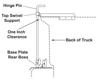
NOTE: The pins must be vertical and the bracket bosses must be aligned with each other. Any misalignment will create difficulty in removal of the pins. Use shims as required to align parts.
