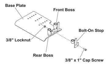
Adjust the base plates and top bracket assemblies to provide at least one inch of clearance between the hinge pins and any point of the truck. The pins must also be positioned vertically.
