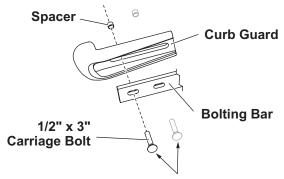
One bolt and spacer for full-length bolting bar. Two bolts and spacers for trimmed bolting bar.  Install the curb guard assembly to the blade (and cutting edge, if present). Reinstall any retained cutting edge washer(s). Add a supplied 1/2" locknut on each carriage bolt. Hand tighten.
