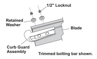
**4. Full-length bolting bar only:** Install a second carriage bolt and locknut using either slot 3 or slot 4. Hand tighten.
