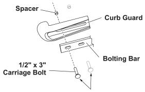
One bolt and spacer for full-length bolting bar. Two bolts and spacers for trimmed bolting bar. 3. Install the curb guard assembly to the blade (and cutting edge, if present). Reinstall any retained cutting edge washer(s). Add a supplied 1/2" locknut on each carriage bolt. Hand tighten.
