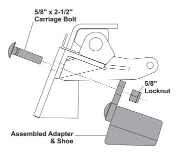
5. Put a locknut on each carriage bolt and tighten to 150 ft-lb.
