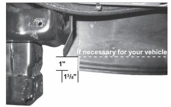
7. Align the holes in the front of the mount with the existing holes at the front of the frame.
