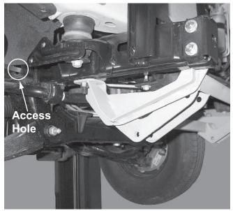
10. Hold the mount tight to the bottom of the frame using a floor jack. Tighten all fasteners according to the torque chart.
