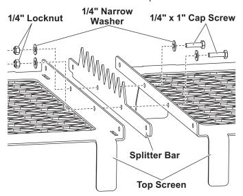
3. Insert the leg of the front splitter latch into the slot in the top screen. Line up the slot in the latch with the splitter bar hole nearest the truck. Fasten loosely using one 1/4" x 1" cap screw, two 1/4" narrow flat washers and one 1/4" locknut.
