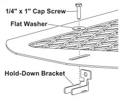
6. Place the screen assembly over the top of the spreader tub. Push the front and back latches toward the tub until legs slide under edge of the tub. Tighten both fasteners. Push the side hold-down brackets toward the tub until the legs slide under the edges of the tub. Tighten both fasteners.
