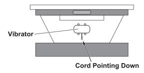
5. Install the vibrator and backing plate with four 3/8" x 2" cap screws and 3/8" locknuts. The vibrator must be installed with the cord pointing down. The vibrator backing plate must be installed on the *inside* surface of the hopper, as shown.
