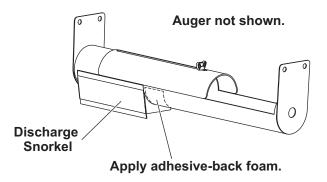
11. Insert the assembled auger tube into the hopper trough with the discharge snorkel extending through the cut-out in the bottom of the trough. Make certain that both ends of auger shaft are reseated in their original positions.
