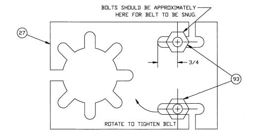
sheave (25) onto pump shaft using locknut and key supplied with pump.
