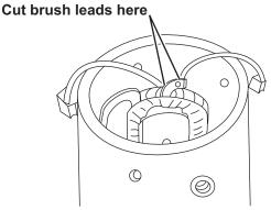
6. Using the furnished hardware, attach the tab in the middle of the two loose replacement brushes to the hole in the field winding tab. Install the machine screw through the brush tab and then through the field winding tab hole. Secure with the external tooth lock washer against the field winding tab and nut.
