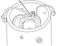
NOTE: The brush tab must have the wires below the screw head. Gently bend the field winding tab away form the motor frame to provide 1/8" clearance. The field windings and brush tab screw or wires must not touch the motor frame or armature, when installed.
