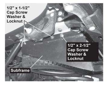
5. Tighten all fasteners according to the torque chart.
