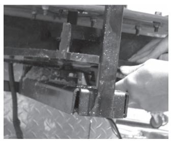
4. Reinstall the belt on the drive and spinner pulleys.
