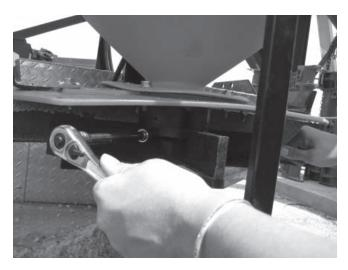
8. Slide the shaft upwards and remove the old spinner.
