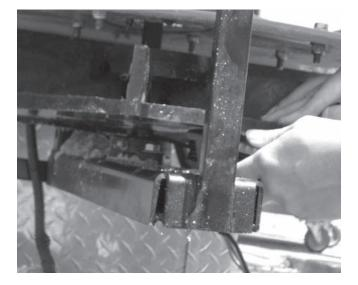
7. Remove the fastener holding the spinner in place.
