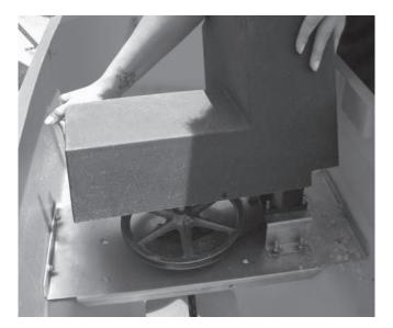
3. Loosen the motor mount fasteners to relieve belt tension.
