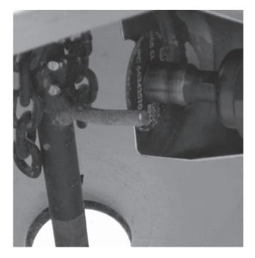
2. Reinstall the locknuts on the upper bearing flange fasteners.
