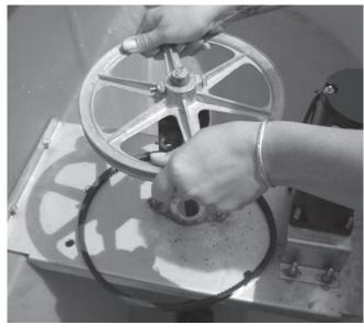
9. Return the old spinner with the deflector rod according to directions received in the service bulletin.
