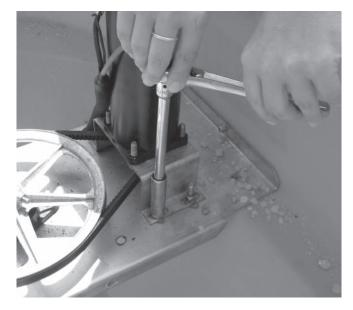
4. Remove the belt from both the drive and spinner pulleys.
