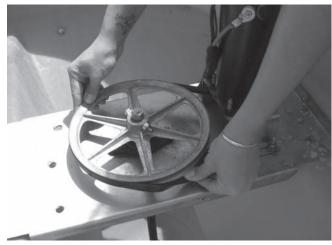
5. Remove the locknuts from the bearing flange
