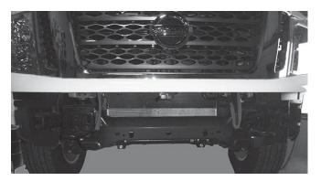
3. Remove and retain the driver-side, passenger-side, and lower plastic radiator shrouds.
