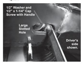
10. Insert a handled 1/2" x 1-1/4" cap screw into the hole found on the inside of the frame behind the radiator. Insert the cap screw in the closest front hole of the mount. Secure with a locknut. Hand tighten the fastener.
