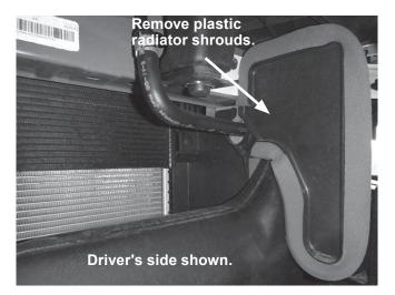
4. On the driver's side, remove the bumper brace and compatibility structure. Save for reinstallation. Repeat on the passenger's side if your vehicle is equipped with a passenger-side compatibility structure.
