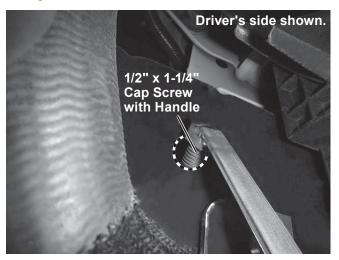
11. Insert a handled 1/2" x 1-1/4" cap screw into the hole found on top of the frame at the front of the vehicle. It may to necessary to trim the handle. Insert the cap screw into the remaining front hole of the mount. Secure with a locknut. Hand tighten the fastener.
