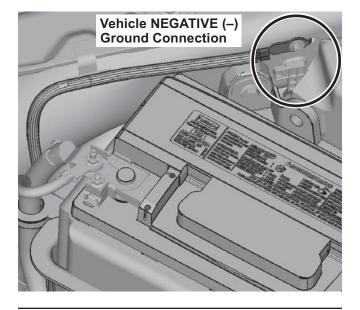
NOTE: Do NOT route the black vehicle battery cable wire to the NEGATIVE (–) battery post. See the Battery Connections section on page 11 for more information.
