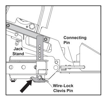
On driver's side, pull up slightly on headgear to relieve pressure on connecting pin while removing the pin. Rotate pin and insert into hole in headgear.
