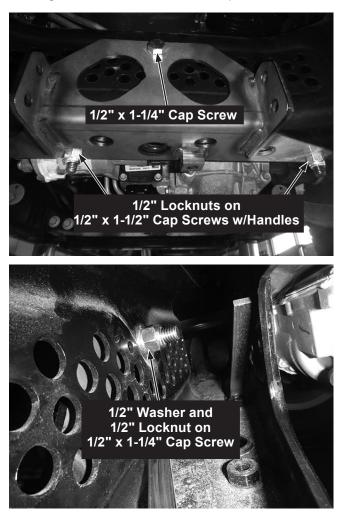
14. With the help of another person, reinstall the bumper. Trim the plastic air dam as necessary to install the mount beam between the passenger-and driver-side hanger assemblies. Insert 1/2" x 1-1/4" cap screws through the hanger assemblies and the mount beam (8 total). Secure each fastener with a 1/2" locknut. Hand tighten.
