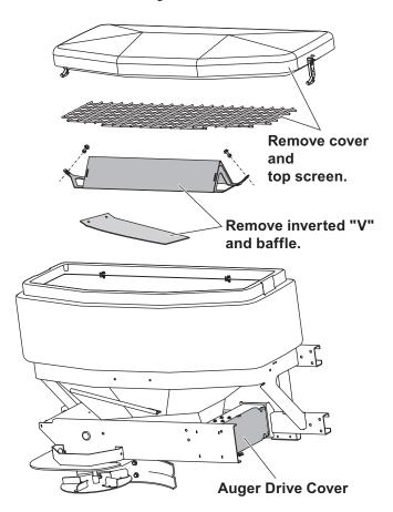
3. Remove the auger and spinner drive covers. Set the covers and all associated hardware aside.
