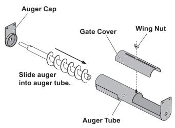
2. Install the motor and gearbox back into the frame. Be sure the auger is seated properly in the spinner side bearing so the set screws can be tightened. The gearbox output shaft will slide into the auger as before. Install and tighten hardware to the gearbox and frame to finger tight. Make sure the auger set screw is on the flat of the gearbox output shaft and tighten down. Once the auger set screw is fully tightened, tighten the gearbox mount bolts according to the torque chart.
