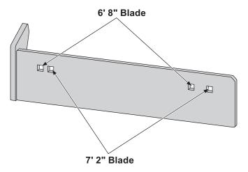
5. Install the curb guard to the blade using two carriage bolts and locknuts. Hand tighten.
