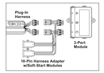
2. Mount the soft-start modules in an area that receives good airflow, such as the cavity between the grille and the radiator.
