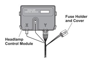
Remove the jumper fuse from the fuse holder and re-insert it in the desired mode position as shown below. Replace the fuse holder cover.
