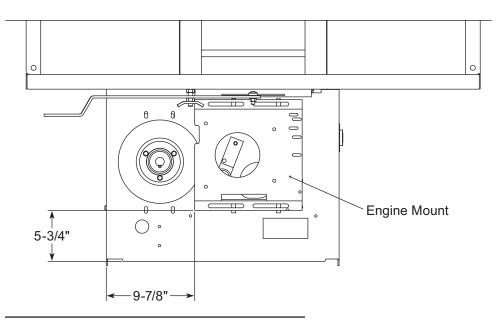
NOTE: Shown with engine removed for clarity.
