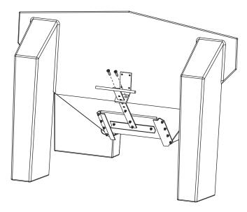
2. Completely remove the feed gate assembly from the spreader by pulling it free of the feed gate guides.
