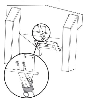
NOTE: Replacement feed gate handle guide should be installed underneath the feed gate bracket.
