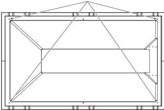
Repeat on all four corners. If needed, remove material at edge of hole with a de-burr tool or a knife so that the repair plate will sit flush on the hopper body.
