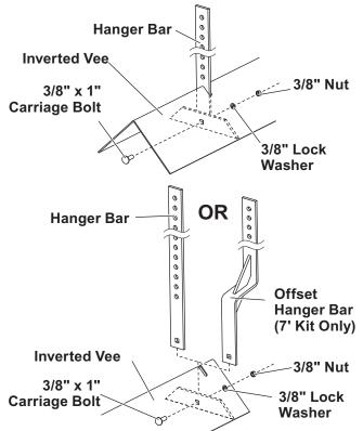
3. Position the vee in the hopper with the longer end towards the chute, as shown.
