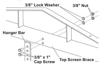
5. If the inverted vee needs to be adjusted higher than this, the hanger bars may need to be shortened to avoid interfering with the closed lids.
