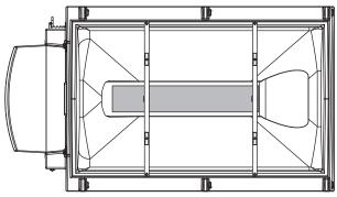
4. Assemble the hanger bars to the top screen brace as shown below. This is an initial inverted vee height adjustment. Final adjustment will depend on the type of material being spread.
