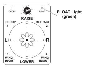
Moving the control lever straight up and down or from side to side on the control body will result in the blade movements described in the following table.
