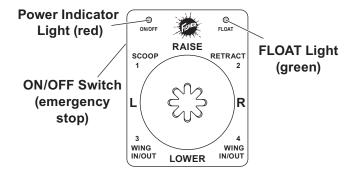
Positions numbered 1, 2, 3, and 4 control SECURITY GUARD™ system functions.
