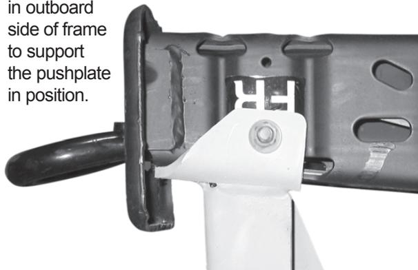
8. Install, but do not tighten, the remaining two tow hook fasteners.
