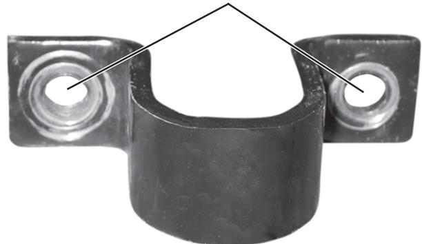
6. Install the bumper mounting bracket to existing frame holes using the self-tapping screw, and the 1/2" x 1-1/2" cap screw with handle, flat washer and locknut. Use only the rear-most holes in the bracket. Tighten these fasteners at this time, then install nutclip taken from BlockerBeam.
