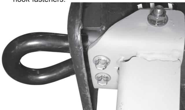
9. Insert the sway bar spacer between the pushplate and sway bar bushing. Loosely attach rear of pushplate using cap screws (1/2" x 1-3/4" in rear hole and 1/2" x 2" in front hole), one flat washer on top of sway bar bracket and one on bottom of modified U-bracket and locknuts. Cap screws and washers may be installed up from below with nuts and washers on top of sway bar bracket as required for clearance.
