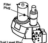
J. Move the control lever, as indicated on label, to control the plow. Raise and lower plow several times to remove air. Recheck fluid level according to Step H.
