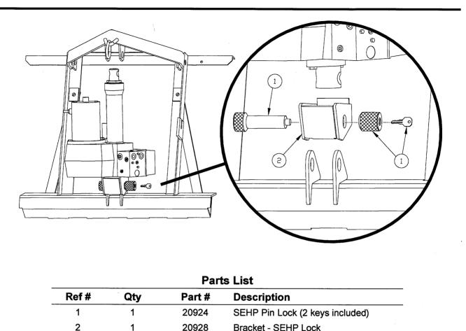
Protect your valuable MINUTE MOUNT® Hydraulic Power Pak using the SEHP Pin Lock. The locking pin replaces the bottom 1" clevis pin on the power pak. The bracket prevents removal of bottom lug from the unit. This kit will deter theft of your Hydraulic Power Pak. However, no system is 100% effective against theft.
