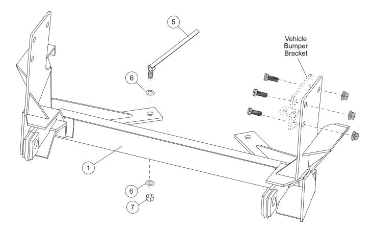
Shaded parts are original vehicle fasteners.
