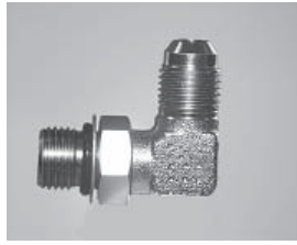
56725 9/16" O-Ring to JIC 90° Elbow
