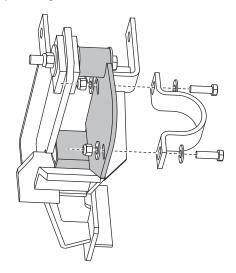
4. Install the ProTube bumper/grille guard into the driver- and passenger-side clamps, and adjust the position as desired. Tighten all fasteners.
