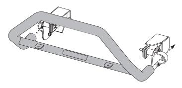
NOTE: After five to ten hours of usage, retorque all ProTube fasteners.
