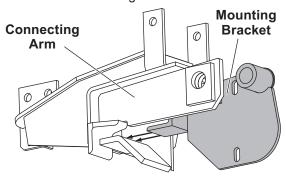
2. Put a 1/2" flat washer onto a 1/2" x 4" cap screw, then insert the cap screw through the holes in the driver-side mounting bracket and the connecting arm. Put another 1/2" flat washer over the end of the cap screw. Place a 1/2" locknut on the cap screw and hand tighten. Leave the 1/2" fasteners loose enough to allow for future adjustment. Repeat for the passenger's side.
