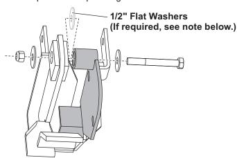
NOTE: The center-to-center measurement for the snowplow connecting arms should be approximately 29-1/8". If the distance is less than that, you may have to insert 1/2" flat washers to eliminate the gap between the connecting arms and the ProTube™ brackets.
