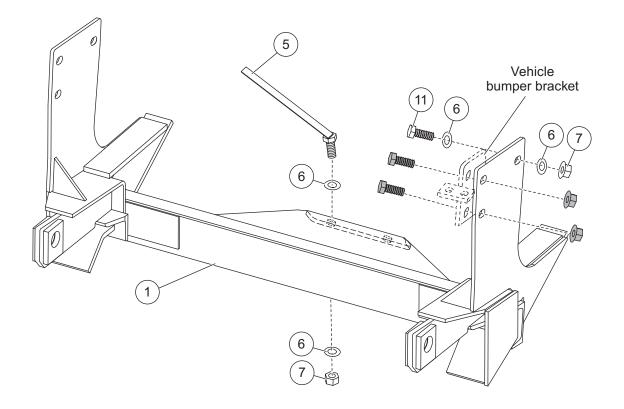
Shaded parts are original vehicle fasteners.
