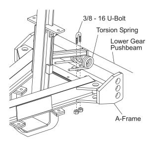
Install Torsion Spring Stop Kit if top hole of A-Frame is used. Do not install otherwise.
