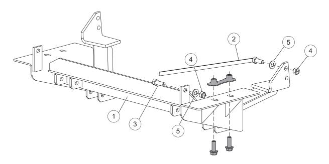
Shaded parts are original vehicle fasteners.
