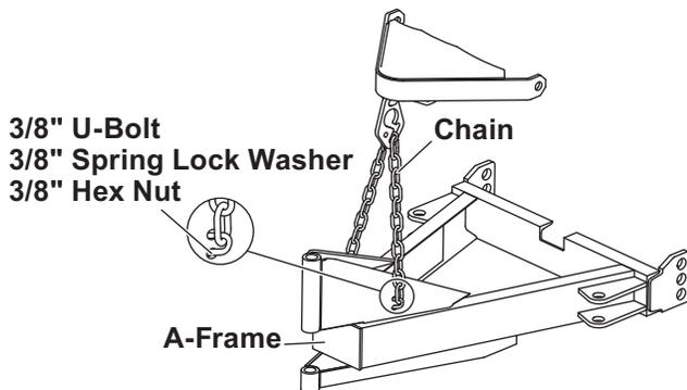
3. Measure from the opposite end approximately 32" and install the second U-bolt to the driver side of the A-frame through the stop link (MM2) or pear link (MM). Set the chain so that, when the blade is raised, the A-frame hits the cross member just before the lift cylinder is fully extended. The lift cylinder should extend 10".
