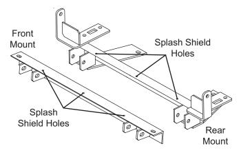
Remove the splash shield, and drill 9/32" holes where marked.
