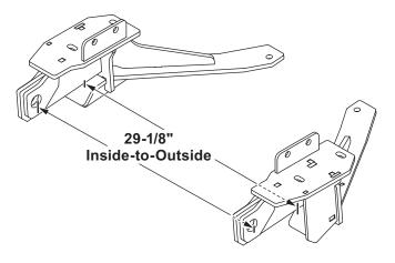
If the measurement is not 29-1/8" and the plates are not parallel, loosen all fasteners and remove the 1/2" x 1-1/2" cap screws holding the tab on the frame for each pushplate. Slide 5/8" flat washers (one for each hole) between the tab and the frame, as needed. Reinsert the cap screws. Tighten all fasteners in the same order as installed.
