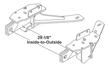
7. Check the inside-to-outside dimension between the connecting pin arms again. Repeat Step 6 as needed to obtain the 29-1/8" dimension while keeping the connecting pin arms parallel.
