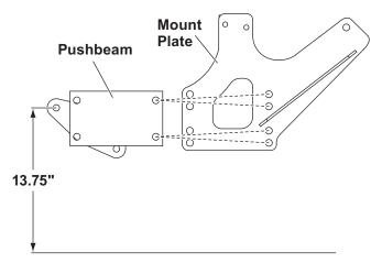
Attach the pushbeam to the mount plates using eight 1/2" x 1-1/2" cap screws (four on each end). Place a 1/2" locknut on each cap screw, and fully tighten according to the torque chart.
